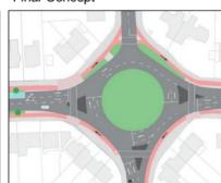
The 'Do Optimum' design promotes the use of a 'Dutch' style roundabout at this junction. While officers agree that this would provide enhanced facilities for pedestrians and cyclists, the modelling of this approach suggests that such a design would severely compromise the vehicular capacity and therefore also have an adverse impact on achieving bus priority.
