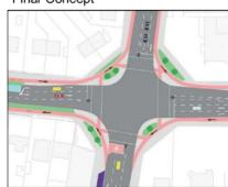
At the King's Hedges Road junction the 'Do Optimum' scheme identifies a preference for a 'Dutch' style roundabout scheme which is what has been modelled within the 'Do Optimum' scenario, within the results show below. However, within the 'Do Optimum' proposals a signalised junction option, with single stage pedestrian and cycling crossing points across each arm has also been identified as acceptable by the LLF.
